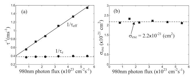
FIG. 5. (a) Measured pulse rise (squares) and fall (circles) time constants of sample A as the function of excitation photon flux. (b) Excitation cross-section derived from the measurement.
