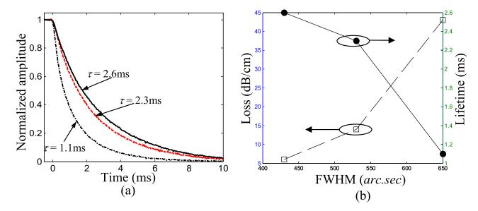
FIG. 2. (a) Measured 1540 nm emission at the falling edge of a pump pulse for samples A (solid line), B (dashed line), and C (dash-dotted line), respectively. (b) Optical loss (open square) and carrier lifetime (circles) as the function of XRD linewidth.
